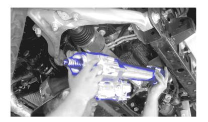
14. Place new rack into chassis from the passenger side. Tilt fore and aft as-required to get pinion shaft to clear differential and engine.
